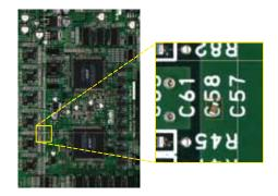
Take advantage of Saki's full PCB scanning by inspecting for loose components, solder balls, and/or foreign materials across the entire surface. Eliminating these defects improves the quality of production while reducing the PPM failure level.
