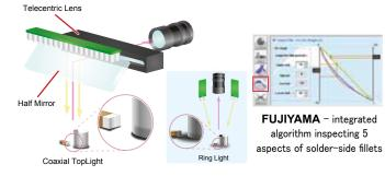
Saki's unique Coaxial TopLight illumination projects light perpendicular to the surface, eliminating shadowing from any objects on the surface. Coaxial TopLight is the best lighting for solder fillet inspection, due to the difference in reflection when a good fillet is formed and when it is not.
