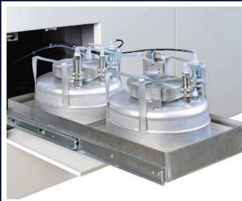
Flux and solder can be added without stopping manufacturing
