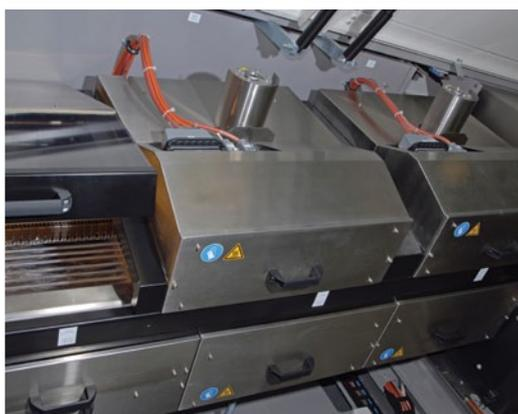
Preheat configurations for process flexibility: IR calrod, quartz lamps, and forced convection
