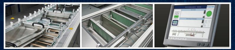
The entire machine (preheater section, solder area and out-feed area) is enclosed in a nitrogen atmosphere. This is monitored in real time by a residual oxygen measuring device and automatically adjusted where required. Adjustment takes place in the PPM range set by the customer in which the processes have been defined. The patented 5-lock (5 flap) system used by the Delta N results in a homogeneous atmosphere throughout the machine and a minimal consumption of nitrogen.
