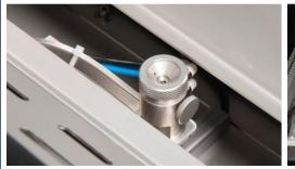
The flux is applied regularly and evenly by means of an atomiser fluxer. The entire closed system is controlled, flux flow rate and level monitoring are both built into this machine as standard. This allows the Delta N to guarantee process stability, even in a 3-shift production.
