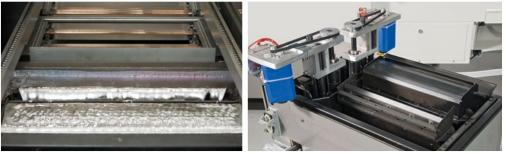
Depending on the machine size, the double wave solder pot contains either 450 or 650 kg of solder (SnPb). The machine is standard equipped with a hollow/chip wave, optional one can add 1 or 2 turbulent waves which can be operated individually. This combination leaves almost no wishes unful-filled and makes it possible to solder all components.
