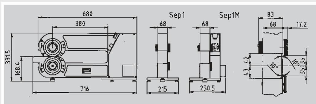
Manual or motorized machine suitable to separate pre-assembled Electronic Board. Precise, reliable and safe. The PCB is manually fed between the lower and upper blades using the scoring as reference. By pushing the board horizontally, the blade rotation starts offering in a sharp and accurate cut. The blade height is adjustable depending on the thickness of the PCB.
