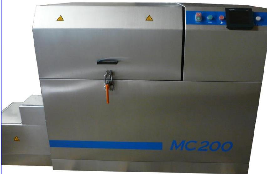
MC200 is based on spray in air technology. Parts are placed into a stainless-steel basket, and submitted to the superior cleaning performance of high flow / low pressure sprayer form 3 Directions while basket rotates. They are perfectly cleaned in just a few minutes.
