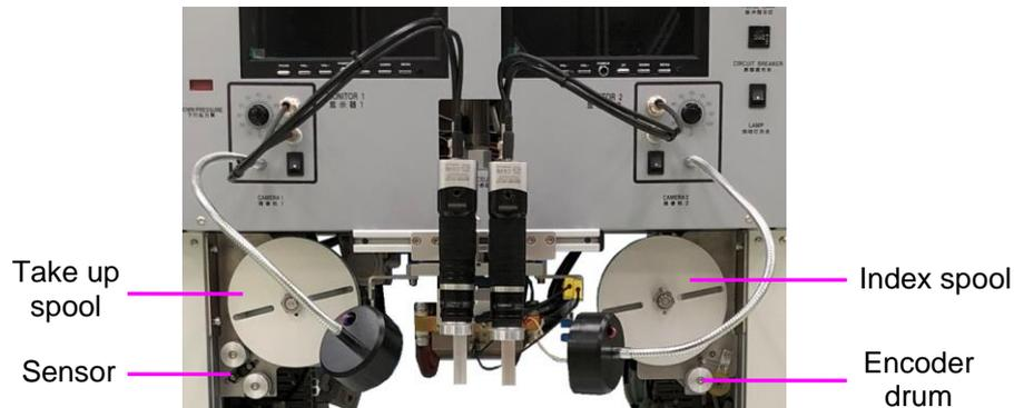
Silicon rubber indexing mechanism is located at the both side of the thermode assembly. A DC gear motor on the right side (Index spool) with a rotary encoder is used to index silicone rubber tape. Make sure that the encoder is free running for more accurate indexing. On the end, take up spool uses DC gear motor which provides tension to spool.
