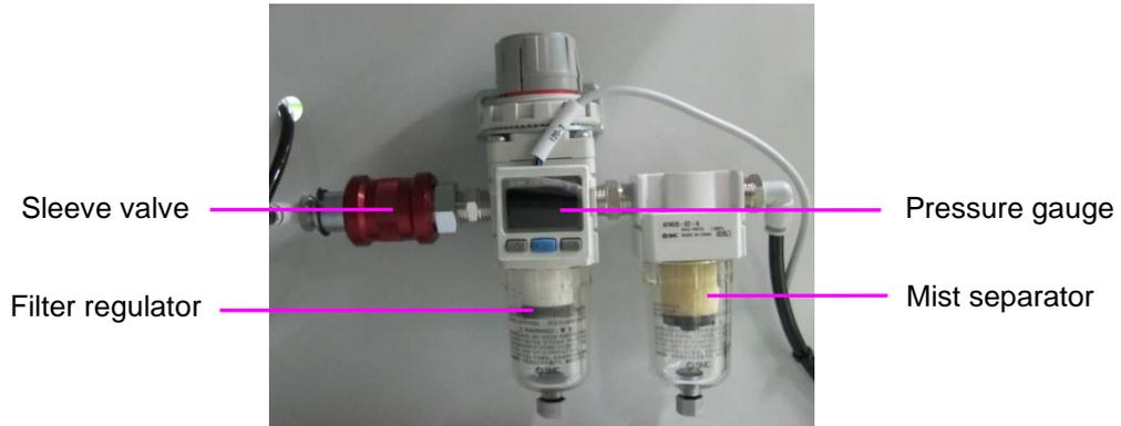
The service unit is mounted at the bottom of the machine. Mainly is used to give dry clean compressed air to the system. A sleeve on/off valve is also connected in line to facilitate setting up.
