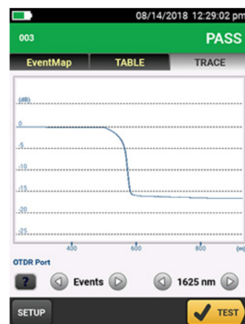
Splitter as seen on an OTDR trace
